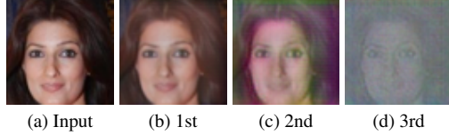
Figure 9. Visualization of the features from different layers of discriminator D using [28]. (a) is the original image. (b), (c), and (d) are the reconstructed results from the first, second, and third convolution layer of D , respectively.
