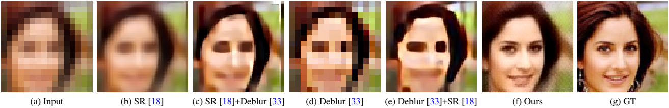
Figure 1. Low-resolution blurry images (a) are challenging for the state-of-the-art super-resolution and deblurring methods ((b) and (d)). Sequentially applying super-resolution and deblurring methods further exacerbates the artifacts ((c) and (e)). Our method (f) learns to reconstruct realistic results with clear structures and fine details. The low-resolution images ((a) and (d)) are resized for visualization.
