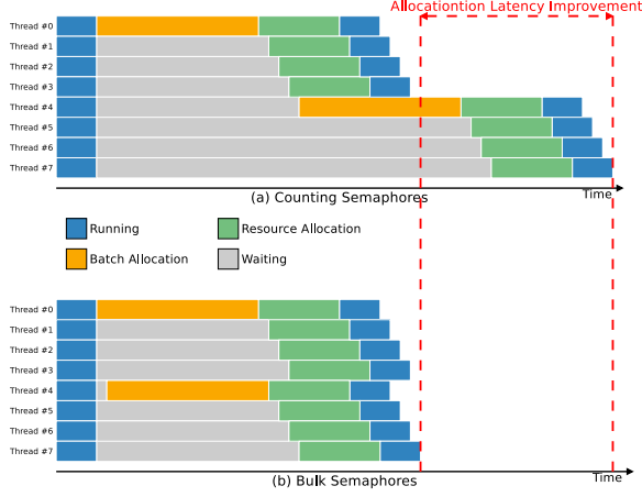
Figure 1. Two-stage allocation example using (a) counting semaphores, and (b) bulk semaphores. In the example 8 concurrent threads use two-stage allocation with a resource batch size of four units.
